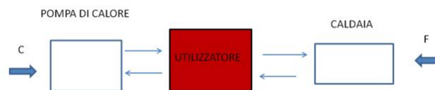
Figure 5.2.9: Configuration HOT7: heat pump and boiler.
